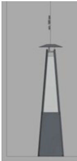
Drawing 6. diagram of minimum safe distance above the heater from combustibile materials.
